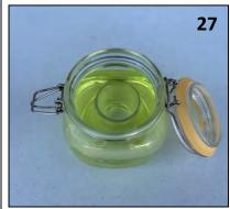
The Sodium Chlorite will begin to react with Hydrochloric Acid to create Chlorine Dioxide.
