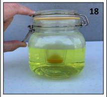
Close and lock Mason jar to avoid losing Chlorine Dioxide gas.
