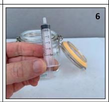
If desired, syringe plunger can be removed to simplify filling. Note, 4% HCl is a weak solution. Hands can be washed when done.
